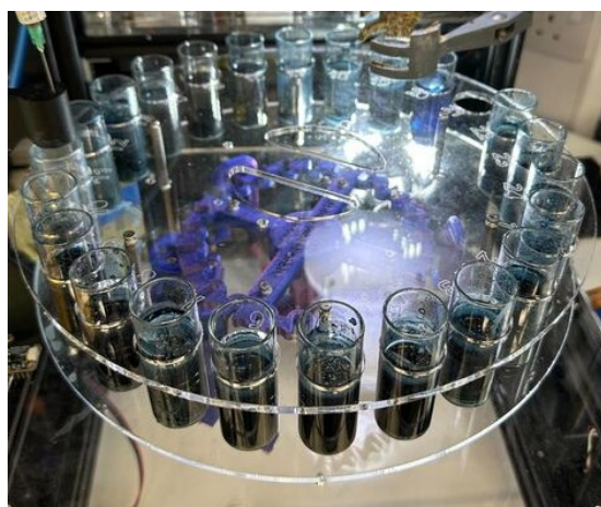
Figure: Photograph of the synthesis wheel in the POM-robot, left and the crystallisation of {Mo 186 } made in the robot
